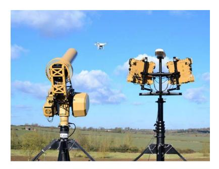
AUDS is a second generation counter UAS system that detects, tracks, identifies, and defeats unmanned vehicles or UAV. The AUDS system is utilizes state of the art radar, precision thermal and daylight cameras, advanced video tracking, and five non-kinetic
