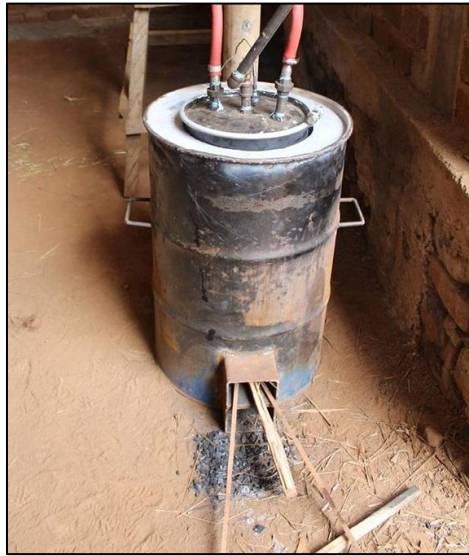
FIGURE 2 2ND GENERATION UKATS BIODIESEL PROCESSOR
